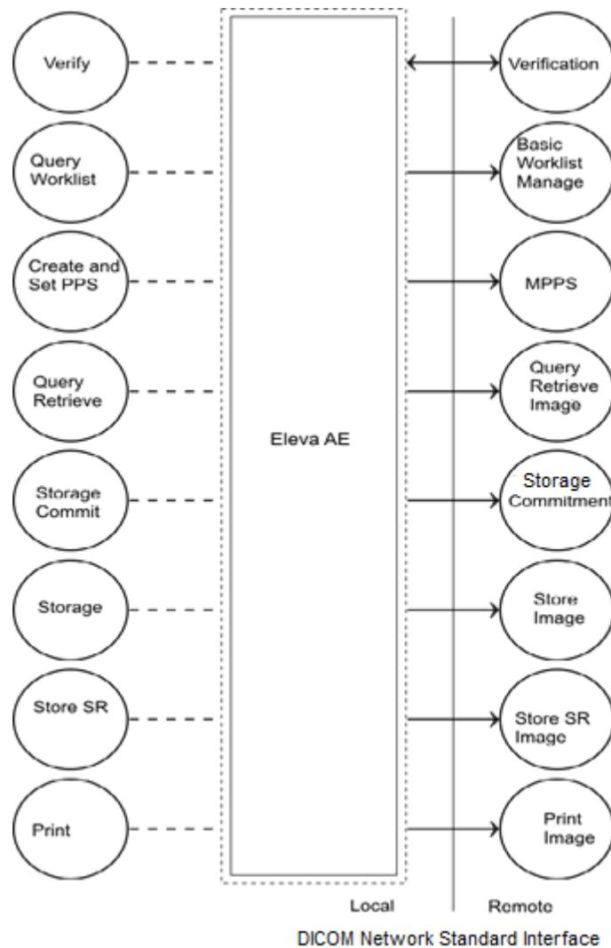
Figure 2: Application Data Flow Diagram
