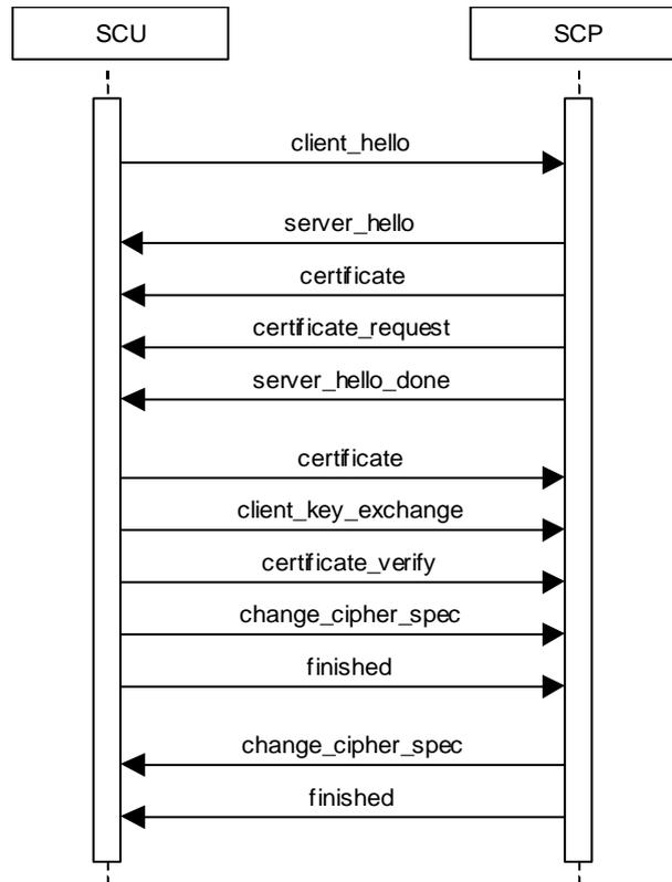
Figure 17: Message flow of TLS handshake
