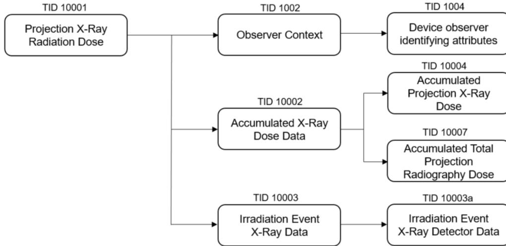
Figure 18: X-Ray Radiation Dose SR IOD Template Structure
